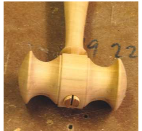
▲ Pic.33 Les has cut a slot in the end of the tenon on the bandsaw. Using a wedge to fix the handle is the traditional way, but Les is planning to use glue as well
